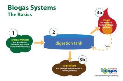
Anaerobic digestion is a four-stage process, sometimes all occurring within one container, sometimes in separate containers, with different bacteria instrumental to each stage.
