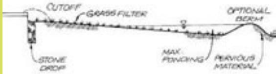
This diagram shows a filter strip designed with a berm to impound water, resulting in improved water quality treatment and increased infiltration. *Image: Center for Watershed Protection*
