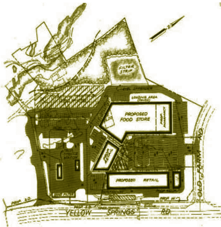
Above: A commercial site design that uses clustering and multiple parking areas to protect water resources and provide opportunities for low impact stormwater management techniques. This design provides the same square footage and parking spaces as a conventional design that encroaches on a nearby marsh (at top.) Image: Center for Watershed Protection
