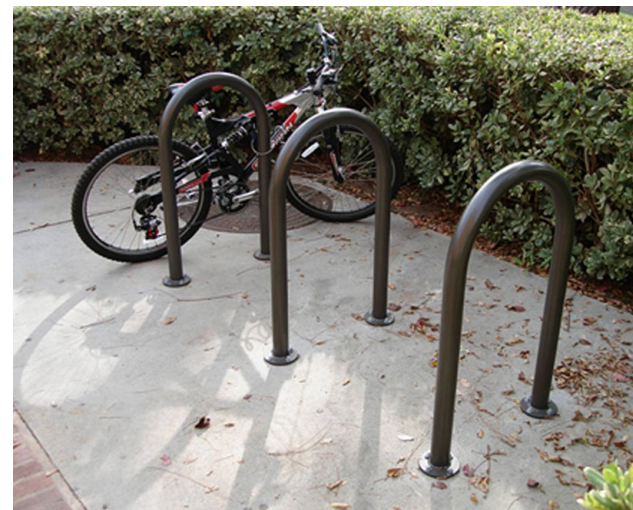
Example of inverted “U” bicycle rack
