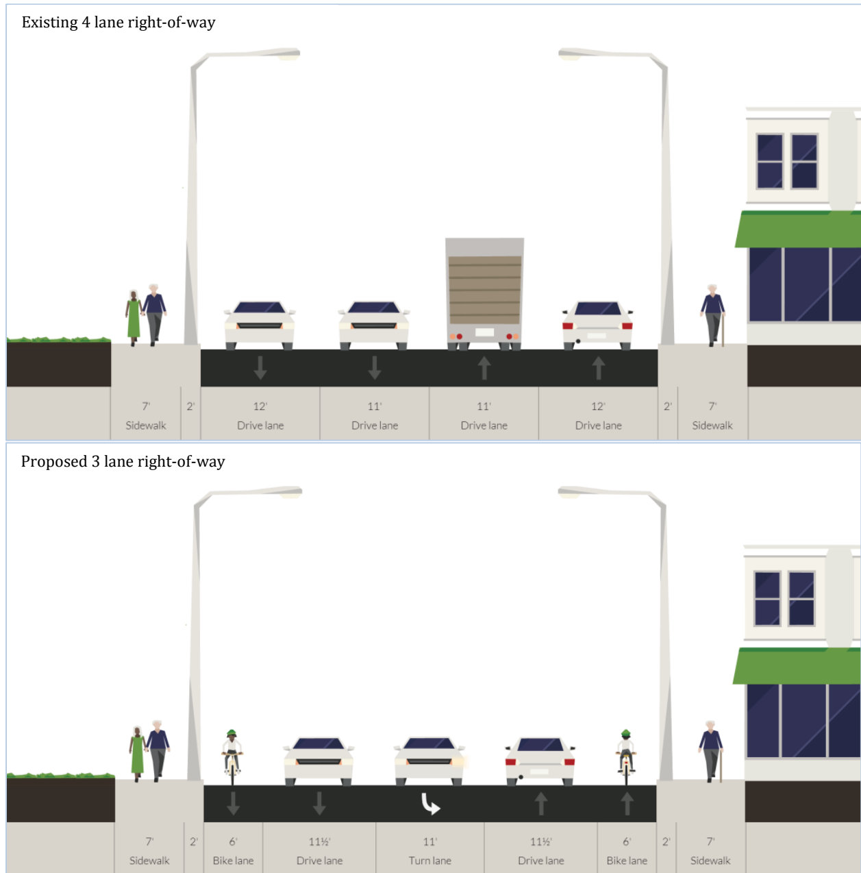
Figure 17: Example of Existing Conditions and Proposed Road Reallocation Hancock Street (between Hunt and East Squantum Streets)
