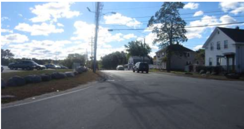
Limited sight distance for Cross Street looking left onto Main Street
