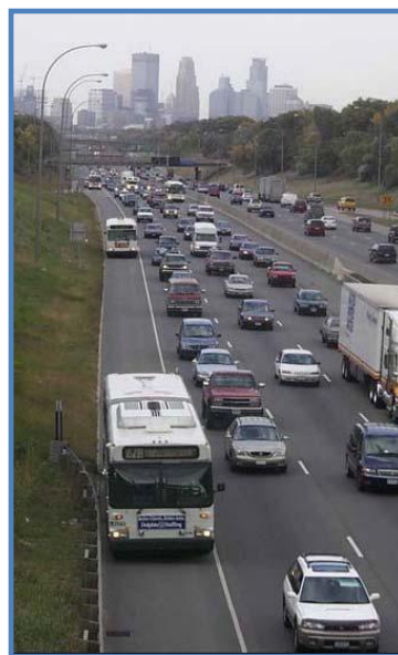
Figure 25 Example of Bus on Shoulder Service
