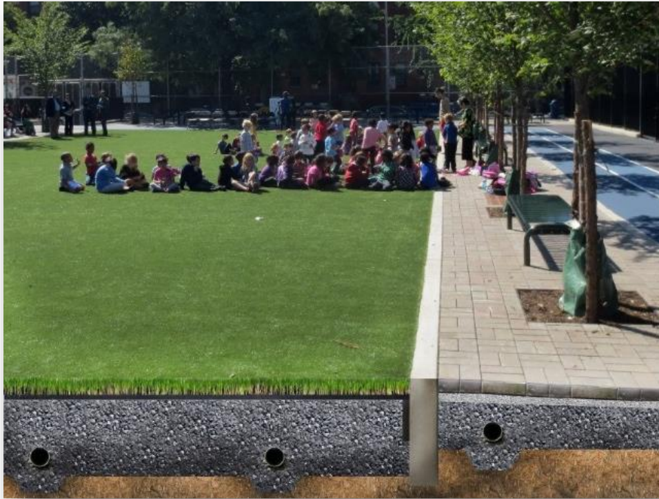
Figure 15 Artificial Turf with Perforated Pipe for Water Infiltration.
