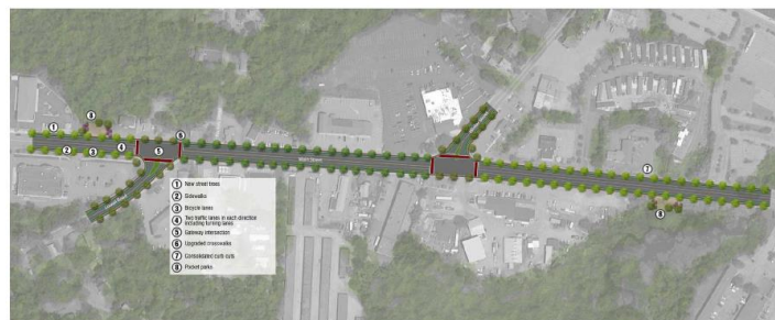
Figure 16: The alternative "Complete Corridor" streetscape calls for maintaining the "T"-shaped intersections, and maintaining two lanes of vehicle traffic in either direction throughout the corridor. Sidewalks would be placed on both sides, with on-street bicycle lanes on either side of Main Street. Aerial source: Google Earth
